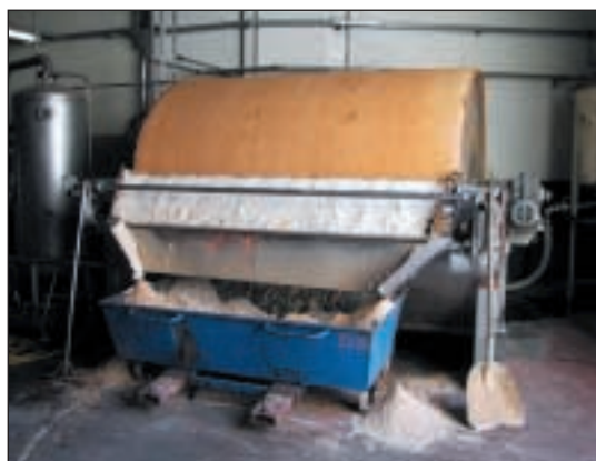
Kieselguhr drum filter for cider at Loïc Raison.
